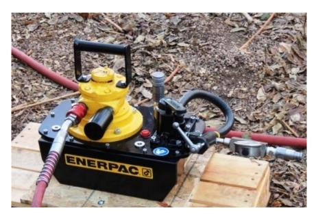
Enerpac ZA-4 Air Drive Hydraulic Pump
