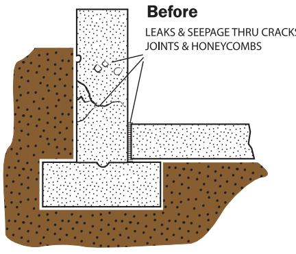
DEFECTS IN FOUNDATION WALLS AND FLOORS PERMIT EASY ENTRY OF WATER FROM SATURATED FILL & GROUND WATER
